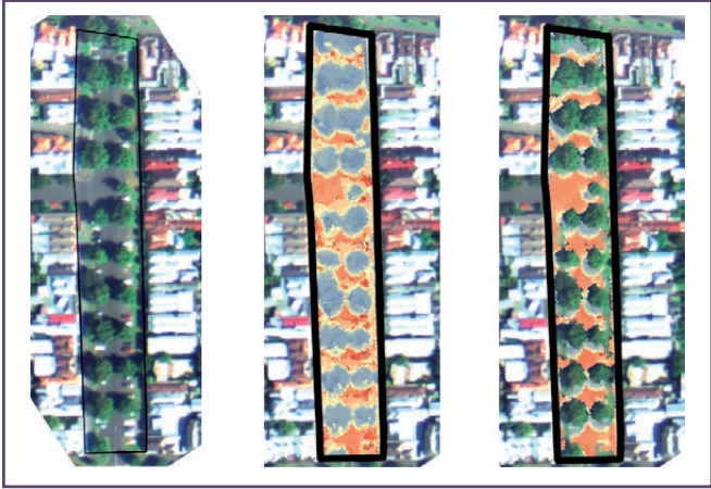
Figure 19: Example of a street canyon polygon (left panel) within the Middle Park focus area. CANYON T_{surf} was the average surface temperature for the whole canyon (centre panel) and the ROAD T_{surf} was the road surface temperature only within the polygon (right panel).
