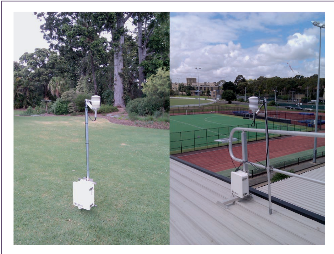
Figure 5: Examples of the ground monitoring sites. Irrigated grass in the Melbourne Royal Botanic Gardens (left) and a rooftop at the University of Melbourne Parkville campus (right).
